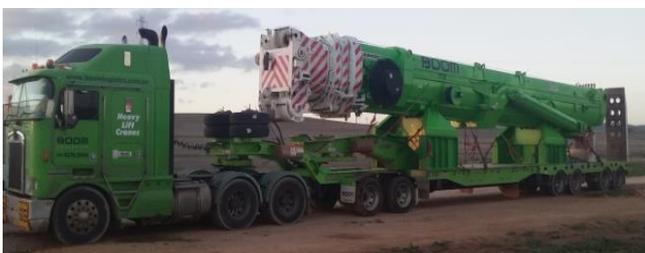
On a straight flat road this does not present a problem, however on corners, its lateral acceleration and high COG present a much greater tipping moment than heavier flat counterweights sitting low on the deck of a trailer. See the photo below.
