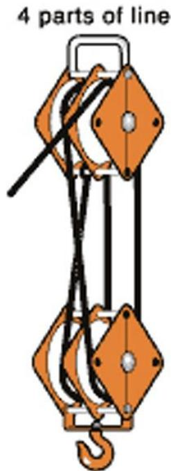
If you only have 2 parts of line in the reeving arrangement, then a 400kg hook block would only be required to keep 200kg rope tension on the drum.
