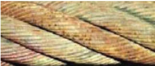
Greasing wire rope will help keep the rope from getting corrosion both on the surface and internally. Several automated grease applicators for wire rope ensure you get sufficient grease without over-greasing. Excessive grease can cause dirt and debris to adhere to the rope and cause premature wear. Greasing an already corroded rope will not remove the existing corrosion.
