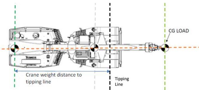
When operating on a side slope, if the load offset goes beyond the crane wheel, the crane tipping line changed to the side wheel line as shown above. In this case, distance between the machine CoG and the tipping line greatly reduced.
