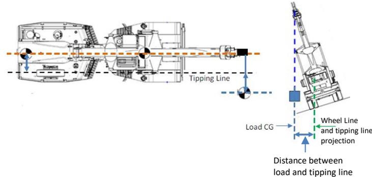
When operating on a side slope in articulated configuration, the crane tipping line changed to the side wheel line. In this case, distance between the machine CoG and the tipping line greatly reduced and distance between the load CoG and the tipping line increased.
