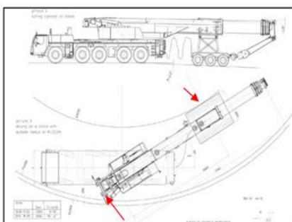
3. The dolly creates up to 50% increase in total length, dramatically reducing the manoeuvrability of the crane.
