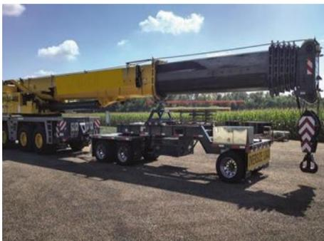
A boom dolly allows heavier cranes to distribute weight over more axles so that the impact on bridge assets and roads are less severe.
