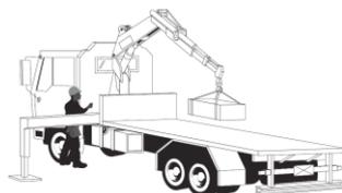
The space available on sites is often constricted. It is frequently impossible to extend all the outriggers of the mobile crane evenly. With the development on crane design, many cranes allow flexible crane outrigger position for crane setup. **But please note that flexible outrigger position is only allowed when specified by the crane manufacture. The specific load chart for that configuration should be used.**
