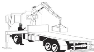
The space available on sites is often constricted. It is frequently impossible to extend all the outriggers of the mobile crane evenly. With the development on crane design, many cranes allow flexible crane outrigger position for crane setup. **But please note that flexible outrigger position is only allowed when specified by the crane manufacture. The specific load chart for that configuration should be used.**
