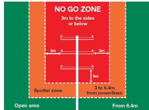
When considering proximity of crane operation, one must be aware that crane operation includes where the crane is set up, but also includes where the load is picked up and where the boom is slewed. If any of these operations got into the *No Go Zone* or the *Spotter Zone*, then effective control measures are necessary.
