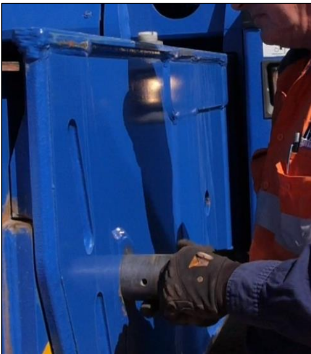
Locking pins should always be used when supplied.
