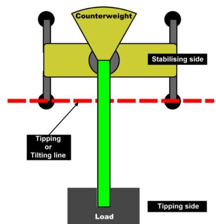
The heavier the load – or the greater the distance the load is from the tipping line (the fulcrum point), the greater the forces are trying to tip the crane over. These forces are counteracted by the weight of the truck & counterweights on the opposite side of the tipping line.
