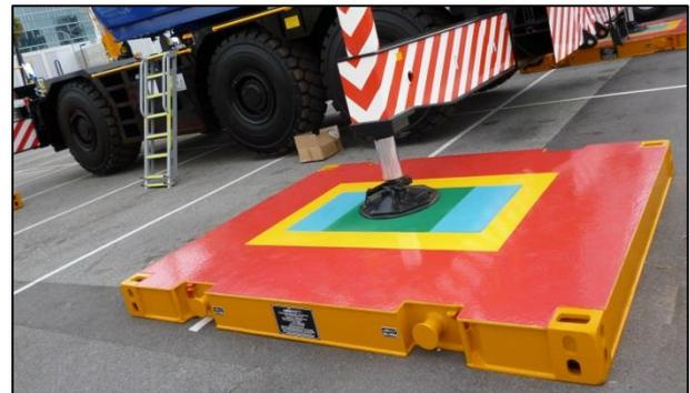
*An example of substantial crane outrigger packing*
